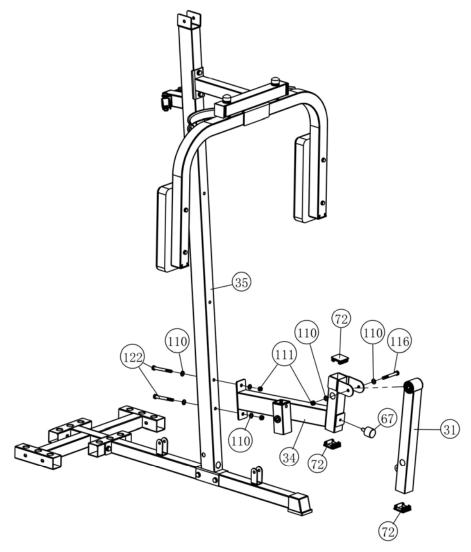
Note: Tighten the bolt (#116) with a wrench to ensure that part (#31) can rotate freely.
