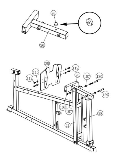
Note: Tighten the bolt (#129, #130) with a wrench to ensure that part (#27, #28) can rotate freely.
