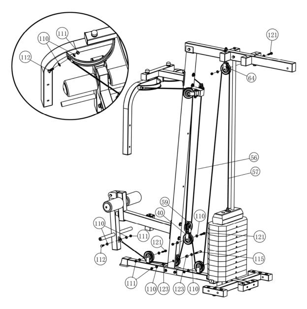
Note: When using a wrench to tighten bolts (#112), do not tighten them too tightly and leave some clearance.
