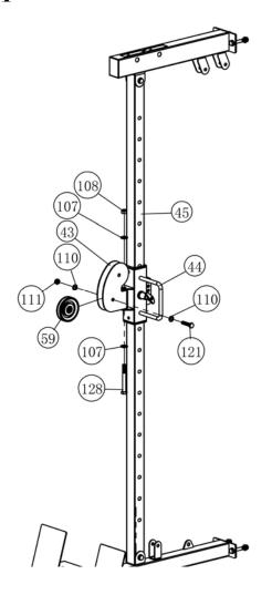
Note: Tighten the bolt (#128) with a wrench to ensure that part (#43) can rotate freely.
