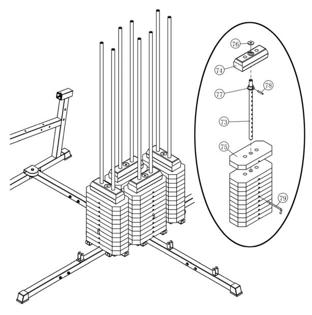
Note: Carefully slide the Weight Plates (#75) one by one onto the guide rods (#63), do not lift more than you can control safely.
